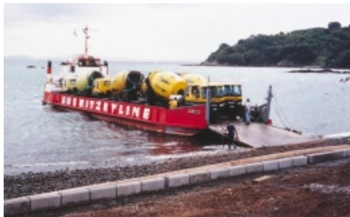
The next 2 days were the busiest with the arrival of 19 concrete trucks, each with 4.5 metres of load. The Port Kennedy made 3 return trips each day, from Gulf Harbour. At one time, there were 6 concrete trucks parked on the road at the entrance to the station.
